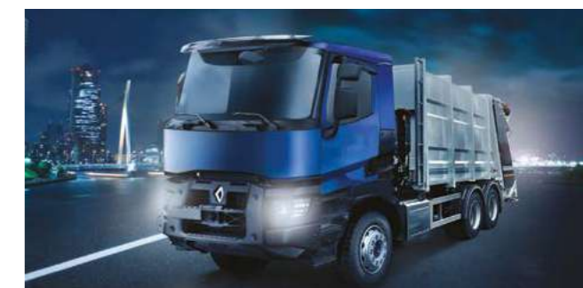
Garbage truck with a hopper capacity of 20-25 m 3
