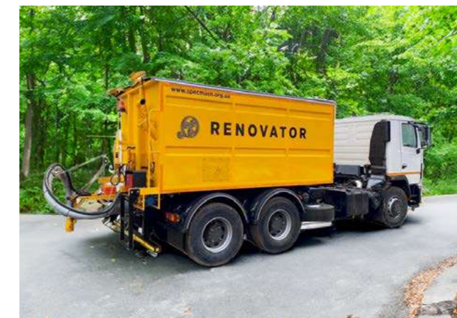
ASPHALT POTHOLE REPAIR TRUCK (RENOVATOR)
