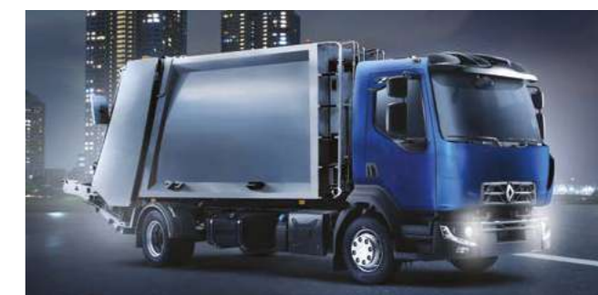
Garbage truck with a hopper capacity of 7-12 m 3
