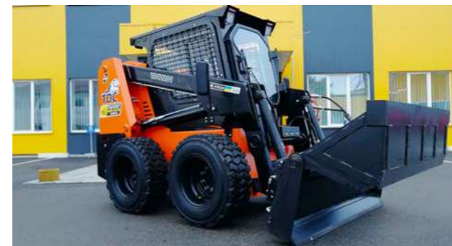
TDC.2.KK.01 Combination Bucket (jaw) for Skid loader
