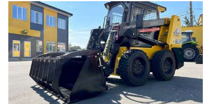
TDC.2.KP900B Clamp Bucket for Skid street loader
