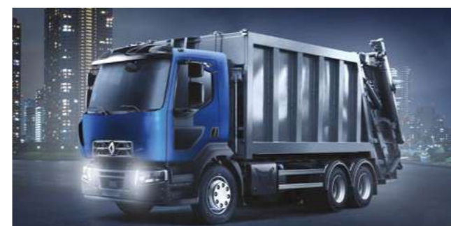
Garbage truck with a hopper capacity of 18-22.5 m 3
